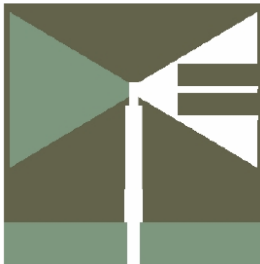
Fig. 2.7: Layout of the double-sided triangular bow-tie antenna on Duroid-5880 substrate [21].
