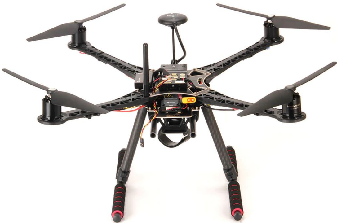
Figure 3.7: Quadcopter frame and components assembly
