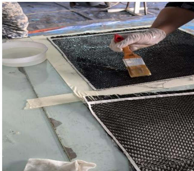
Figure 3.3: Carbon Fiber Frame Fabrication
