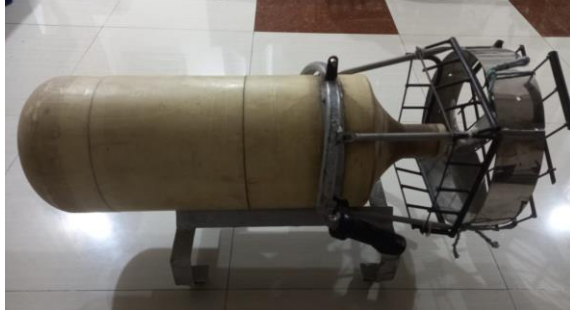
Fig 8.2: Assembly of Mechanical and Electrical component of DPV.
