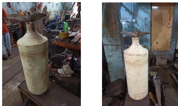
Fig 7.4: Assembly of body and propeller of Diver Propulsion Vehicle.
