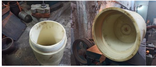
Fig 7.2: External Threading around the body of Diver Propulsion Vehicle.
