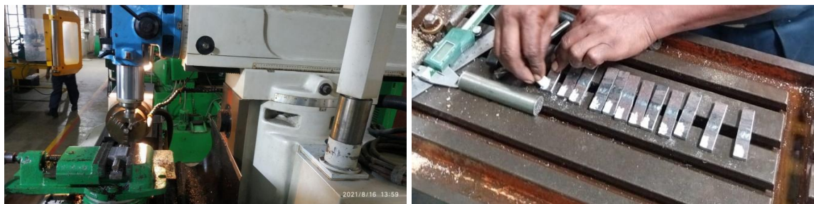
Figure 2.2: Machining of the coupons in the CNC Cutting Machine of BN Dockyard.
