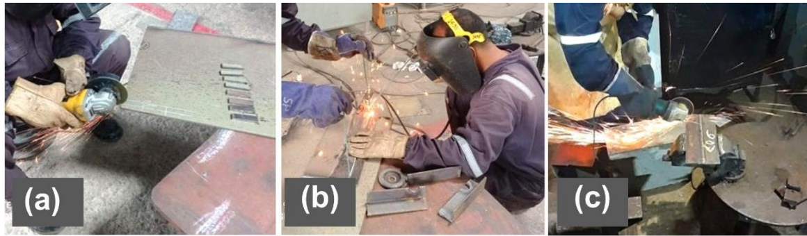
Figure 2.1: Cutting and sizing of the coupons in BN Dockyard Shop: (a) sample cutting, (b) butt welding of the samples, (c) cutting of welded metals
