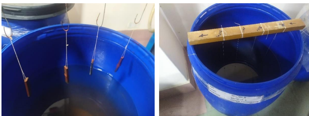
Figure 2.6: Immersion of the metal specimens in the stored seawater for gravimetric analysis
