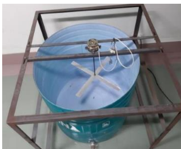
Figure 3.8: Experimental setup for the seawater dynamic lab test.
