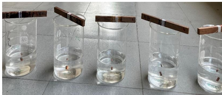
Figure 3.9: Metal matrix composite samples immersed in the 3.5% NaCl salt water solution at room temperature
