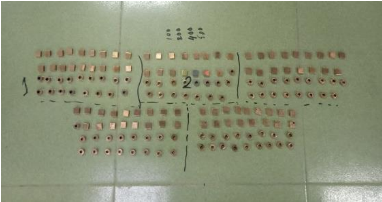
Figure 3.5: Prepared electro-magnetic test samples of the Cu-Al 2 O 3 composite at a glance
