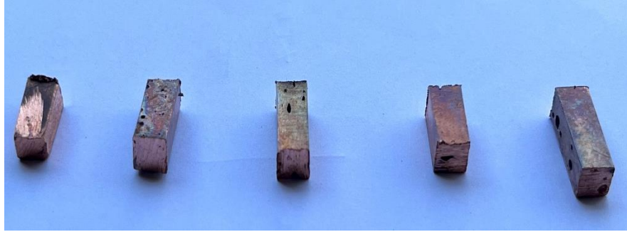
Figure 3.8: Metal-matrix composite samples used for gravimetric corrosion test
