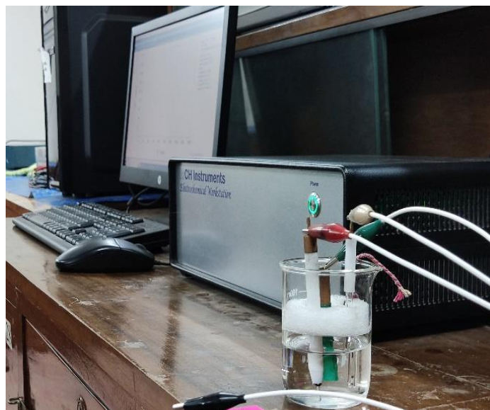
Figure 3.11: CH workstation used for both potentiodynamic polarization and electro-chemical impedance spectroscopy test
