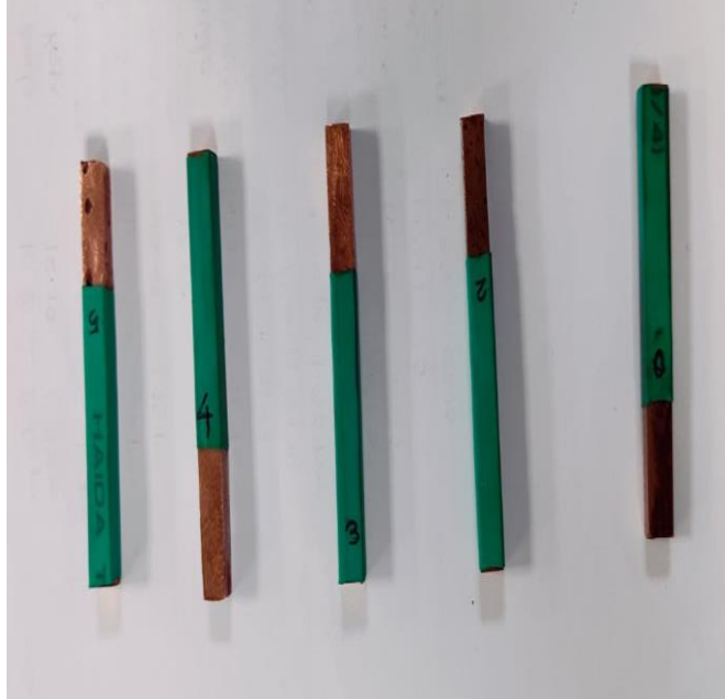
Figure 3.10: Metal matrix composite samples used for electro-chemical corrosion test with the heat shrinkable tube attached with samples to avoid unwanted exposal of surfaces
