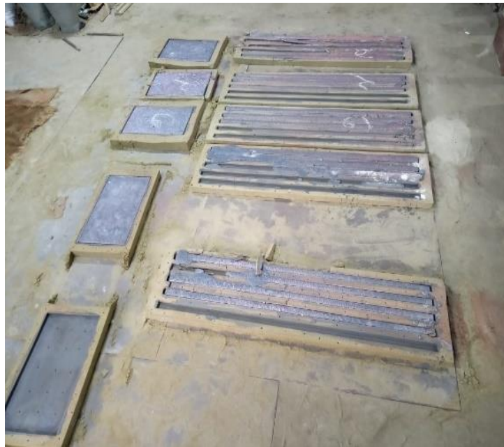
Figure 3.3: Final metal-matrix composite sample (as cast) prepared after natural cooling at environmental conditions
