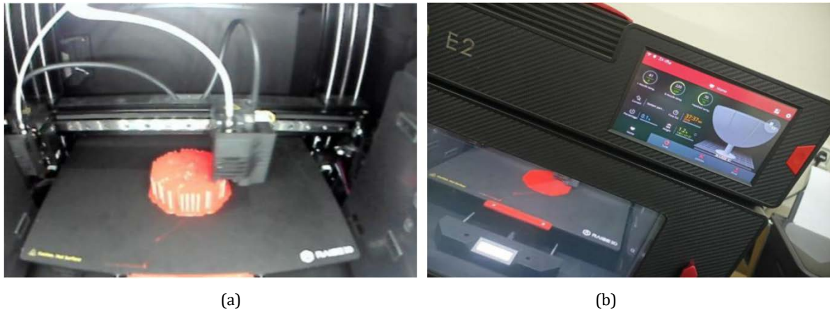
Figure 9: 3D printing of the reflector model on RAISE 3D E2 machine: (a) 3D printing of support structure, and (b) Digital screen of machine
