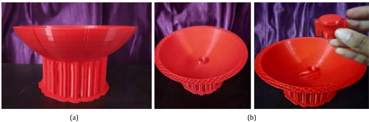
Figure 10: The failed part of the bottom structure of 3D printed spherical antenna (1 st trial), (a) front view and (b) collapsed feed array
