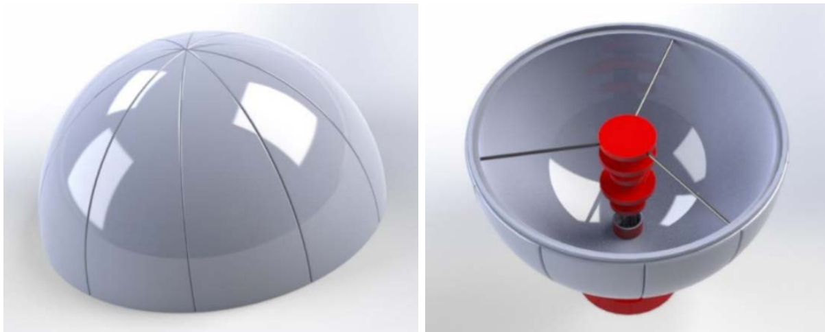
Figure 7: Spherical reflector model design, (a) Upper part and (b) lower part
