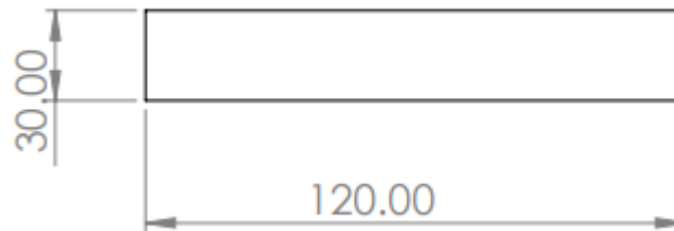
Fig. 4.7: Standard flexural rigidity testing specimen dimension.
