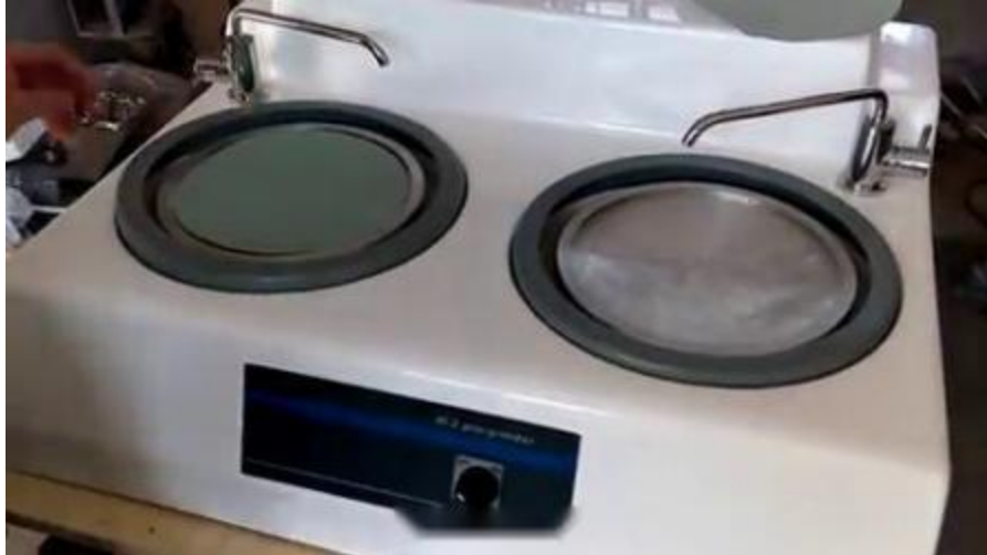
Fig. 4.1: Polishing machine to prepare the composite for etching (NANO 2000T Grinder-Polisher).
