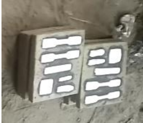
Fig. 3.14: Materials pouring and specimen preparation.
