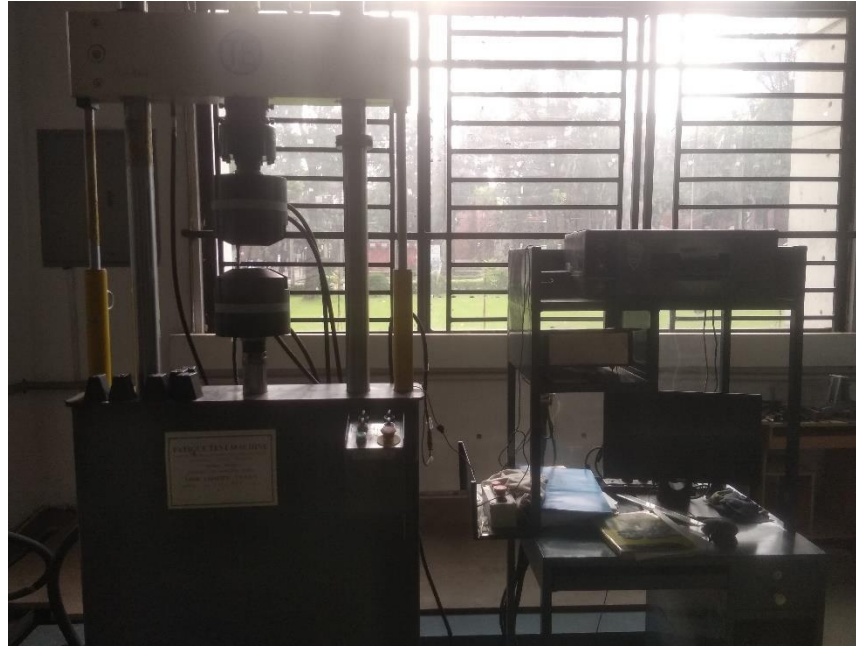
Fig. 4.6: Setup for tensile testing and flexural rigidity testing (Universal tensile tester PLS100).
