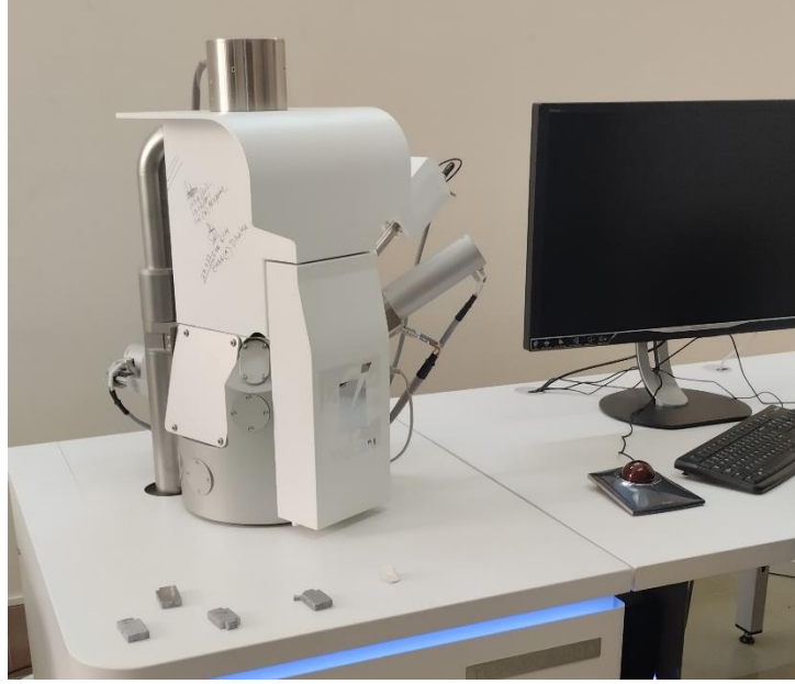
Fig. 4.3: Scanning electron microscope setup (Tescan Vega).
