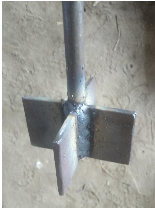
Fig. 3.11: Stirring blade setup (before Boron nitride) coating.
