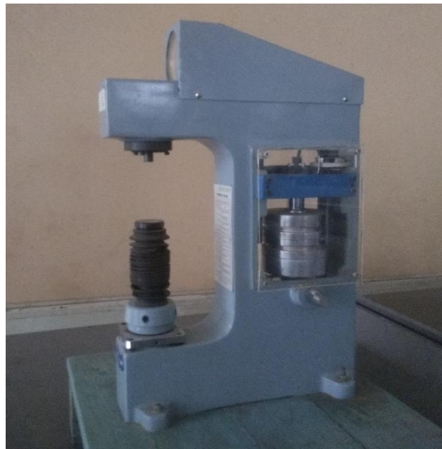
Fig. 4.11: Setup for hardness testing (Brooks hardness tester, RAS).
