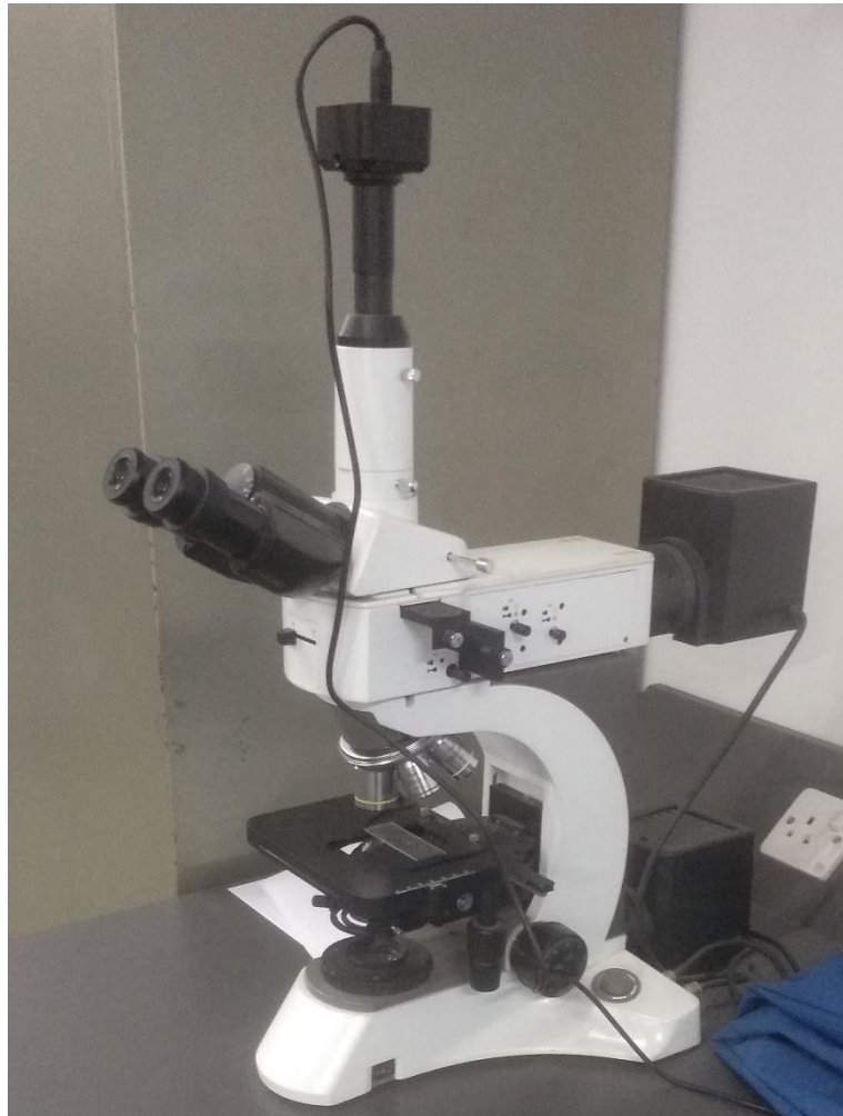
Fig. 4.2: Optical microscopic setup (Laboratory metallurgical microscope BS-6022RF/TRF).
