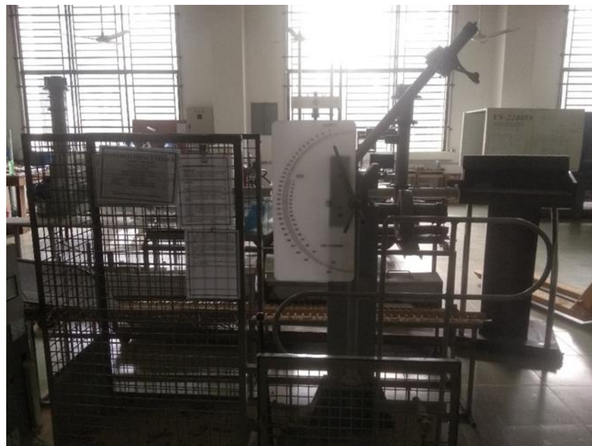
Fig. 4.14: Setup for impact testing (Universal impact tester, AIT3000kN).
