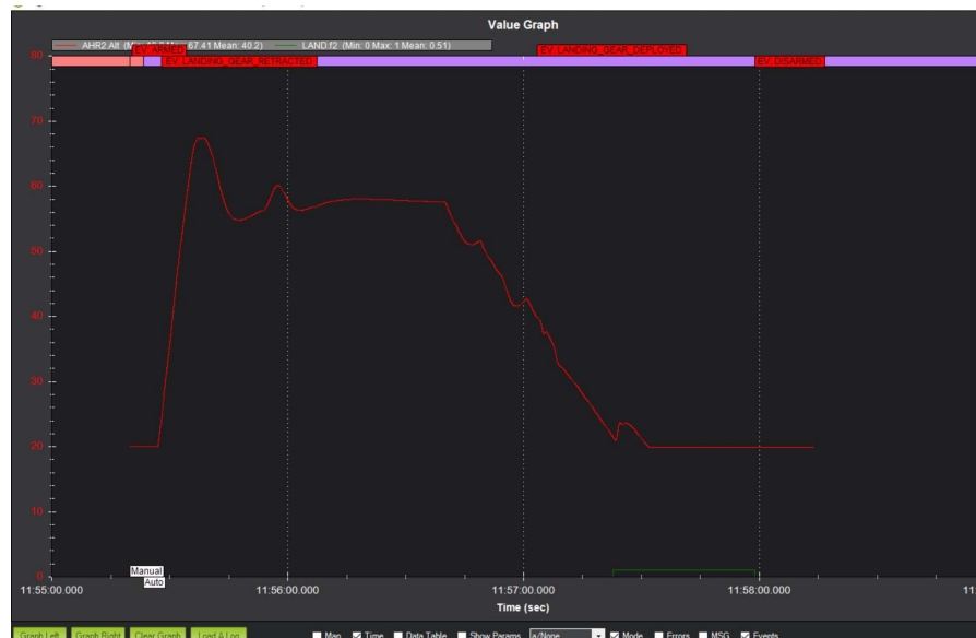
Fig: 4.1 Flight log showing the altitude AGL vs Time
