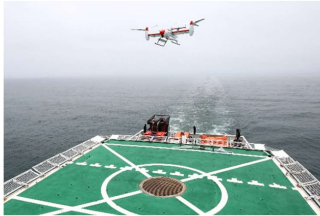
Fig 1.5: Recovery of Tilt Rotor Platform on moving ship using RTK GPS
