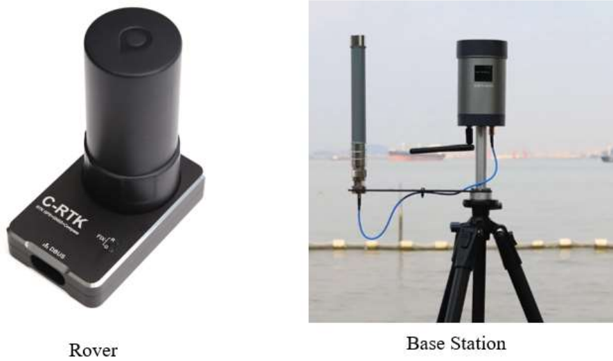
Fig 2.6: Components of RTK GPS Source: www.cuav.net
