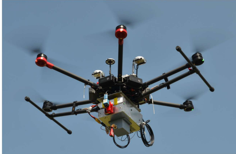
Fig 1.4: Matrice 600 Hexacopter used as test platform for 122 GHz monostatic radar
