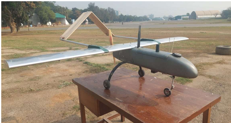
Fig 3.9: The designed UAV for real test flight
