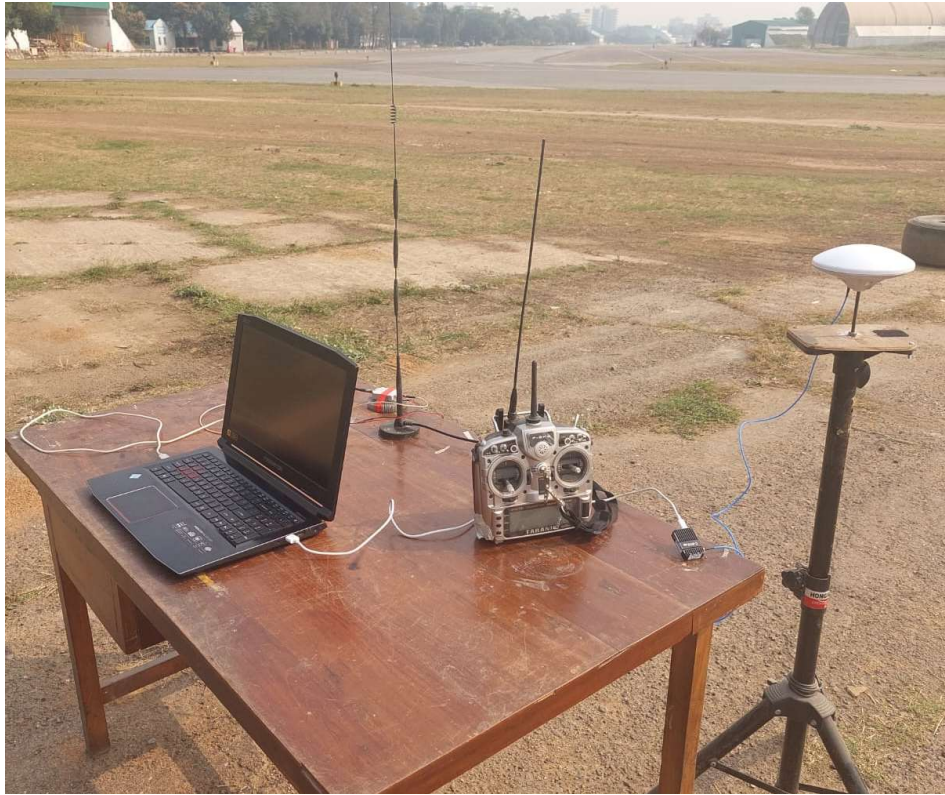
Fig 3.8: RTK GPS and GCS setup for Test Flight
