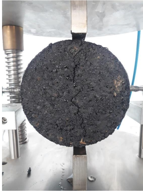
Figure 3.16 Failure of the specimen after ITS test
