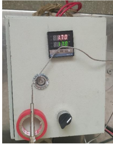
Figure 3.8 Controlling temperature through a thermocouple
