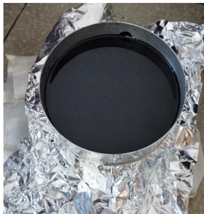
Figure 3.9 PMB stored in a container
