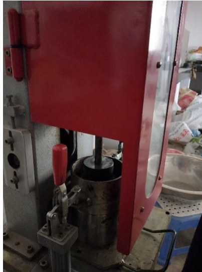
Figure 3.10 Compaction of Marshall specimen using Automatic Compactor
