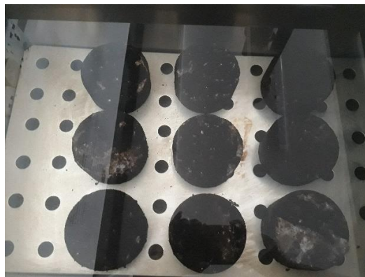
Figure 3.17 Conditioning of Marshall sample in a 60°C water bath
