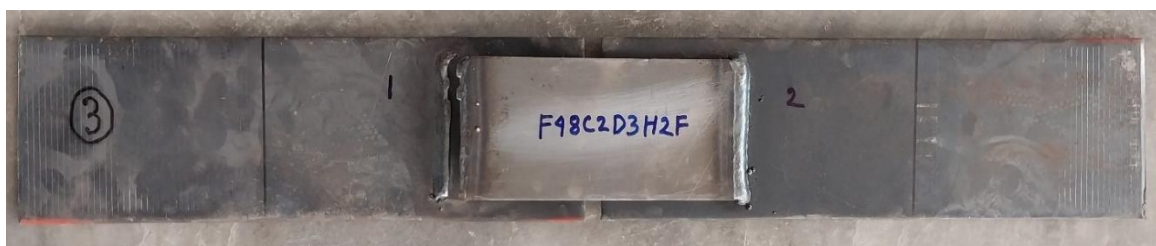
(c) . Weld throat failure (WTF)
