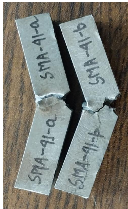
(b).SMAW Welding (E6013)
