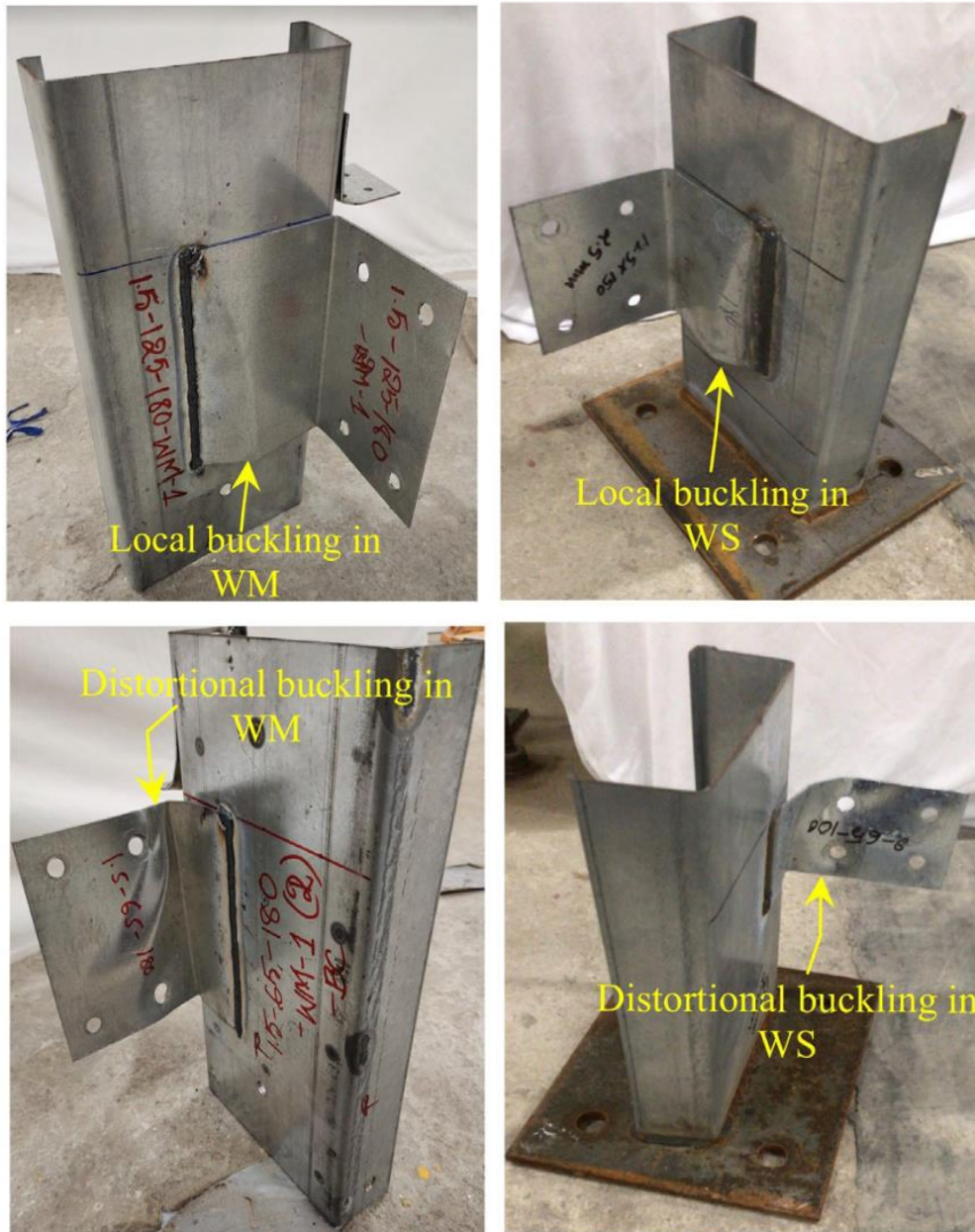
Figure 2.11: Failure modes in WM and WS (a) WM-local buckling; (b) WS-local buckling; (c) WM-distortional buckling; (d) WS-distortional buckling (Mallepogu and Madhavan, 2023)
