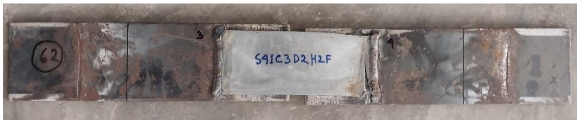
(b). Tearing of plate adjacent to the weld (TPAW)
