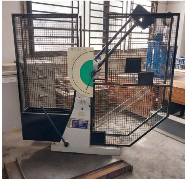
Figure 3.18: Charpy V-notch weld coupon test setup
