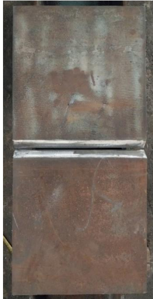
Step-1: Two 25mm thick Plate with 45-degree bevel
