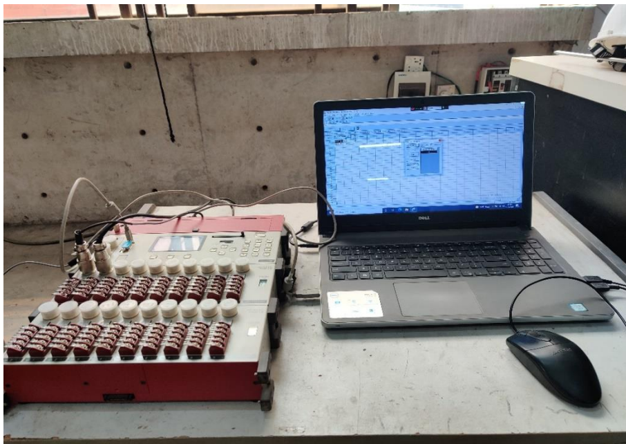
Figure 3.24: Setup for load and elongation data acquisition
