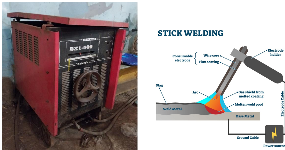
Figure 2.5: Shielded metal arc welding (SMAW) (Sild, 2022c)
