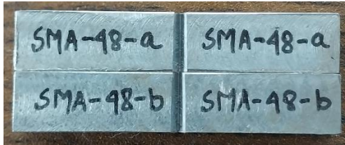
(c). SMA Welding (E7018)
