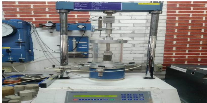
Fig. 3.13: Unconfined compression test
