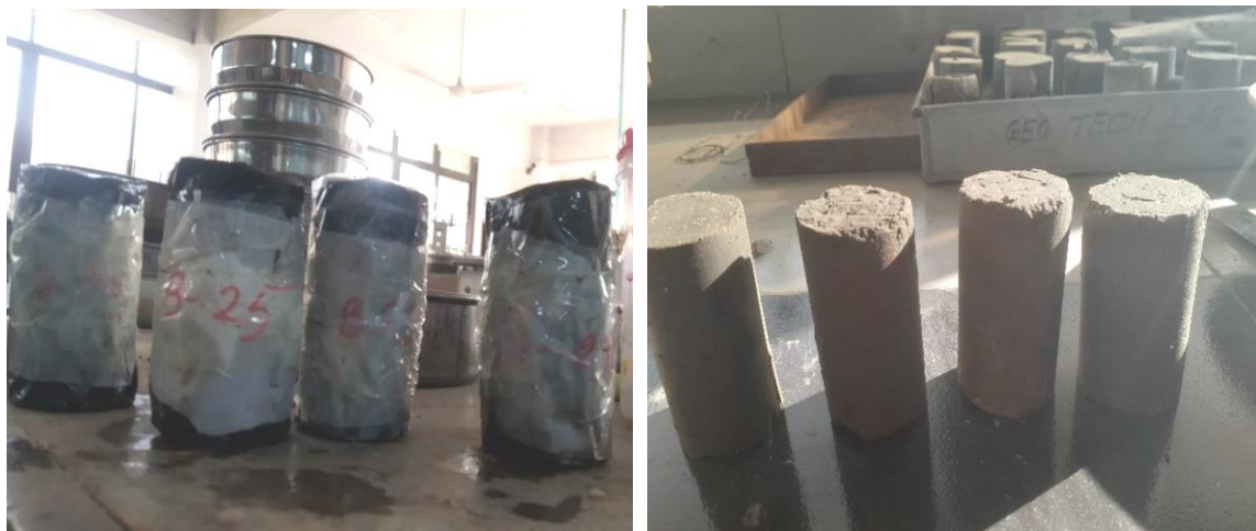
Fig. 3.12: Specimens in ambient condition (a) before and (b) after curing period
