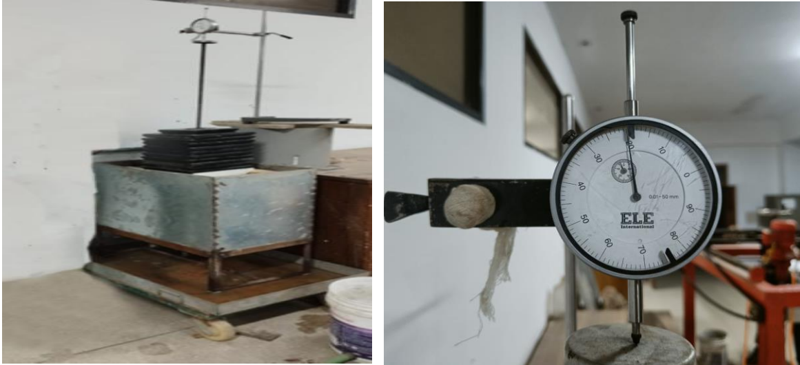
Fig. 3.19: Strain reading monitoring.
