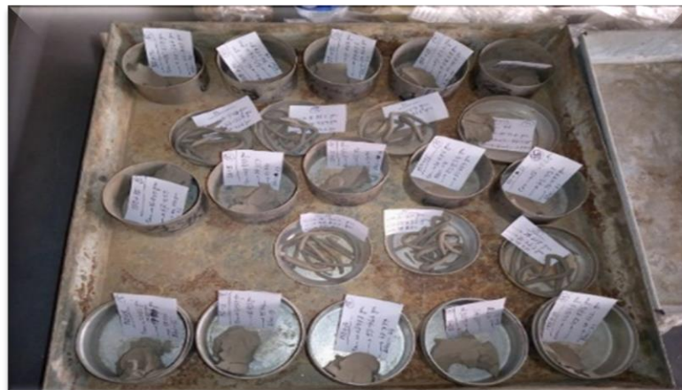
Fig. 3.4: Atterberg Limit Test
