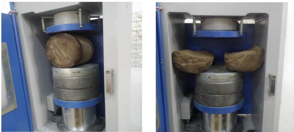
Fig. 3.14: Split tensile test in compression machine.
