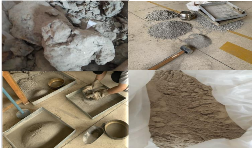
Fig. 3.3: Collected Soil before grinding and after grinding
