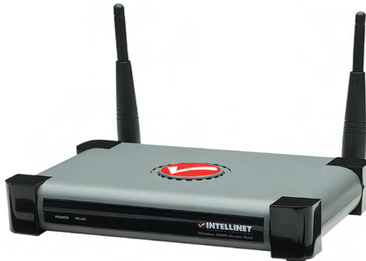
Figure 3.3: wireless 150n access point
