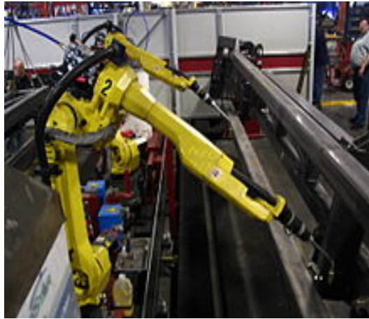
Figure 2.1: Articulated welding robots used in a factory, a type of industrial robot.
