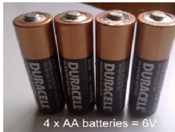
Figure 3.7: 4 AA batteries i.e. 6V for motors and servo
