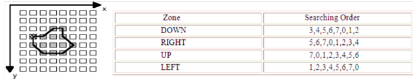
Figure 3.9: (a) Chain code generation for an image, (b) Searching order in the four zones
