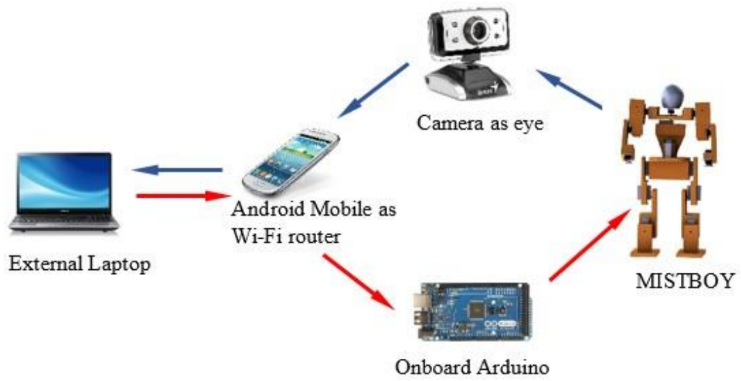
Figure 4.14 Integrated Vision system.
