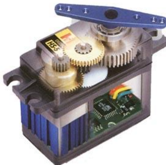
Figure 5.2: Servo motor for rotational movement of arm
