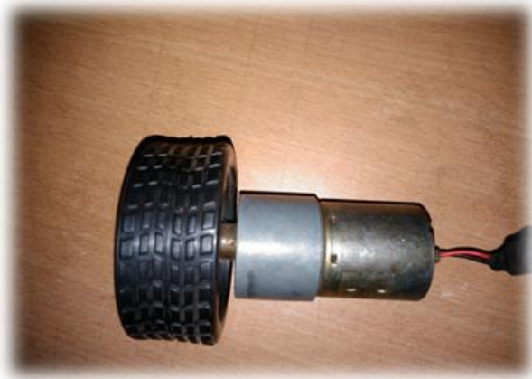
Figure 6.3 : DC geared motor .
