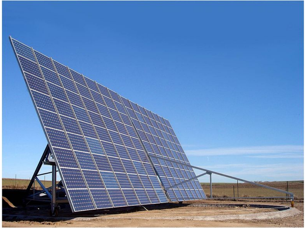
Figure 6.3 :Azimuth-altitude dual axis tracker - 2 axis solar tracker, Toledo, Spain.[39]
