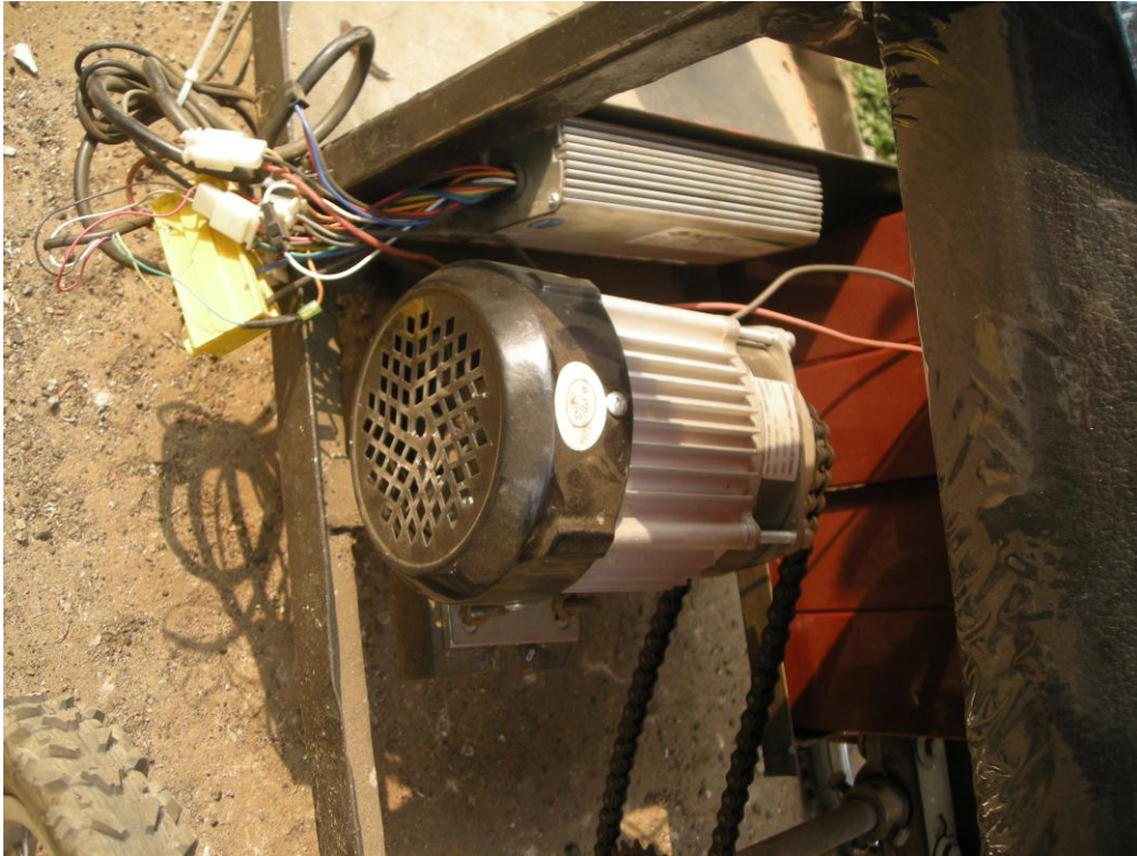
Figure 5.5.4:b. Motor with Control Unit
