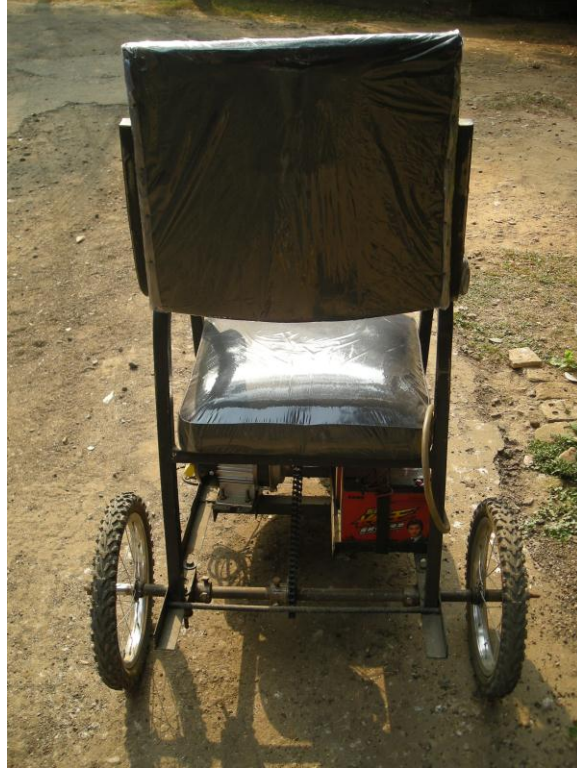
Figure 5.5.2.2 : Main frame (Back view)
