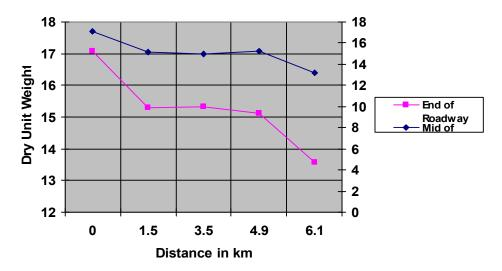
Graph 4.3: Variation of dry unit weight  $(\gamma_d)$  obtained from Standard Proctor Test
