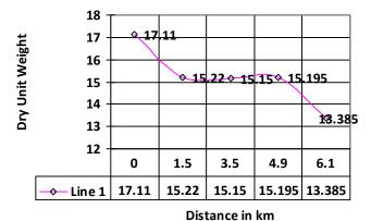
Graph 5.1:Dry unit weight obtained in the field by Sand
