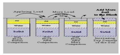
Figure 2.3: Mechanism of soil compaction
