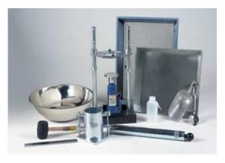
Figure 4.2: Standard proctor test apparatus (geotech.org)
