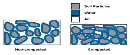
Figure 2.1: Effects of compaction on pore space
