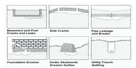
Figure 2.4: Results of poor compaction
