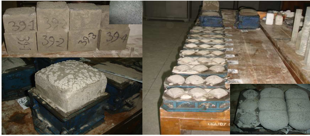
Figure 1: Volumetric expansion in cube sample and voids distribution in mortar matrix
