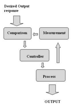
Fig 1: Block diagram of a controller
