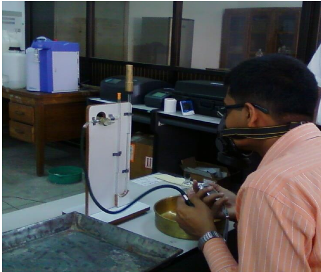
Figure 5: Determination of fineness by Blaine's apparatus
