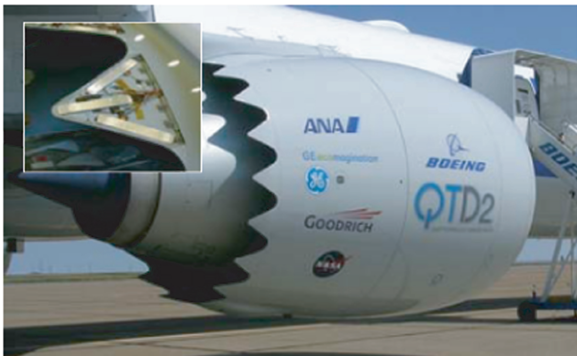
Figure 5: Variable geometry fan chevrons (inset shows individual chevron with cover removed) [15]
