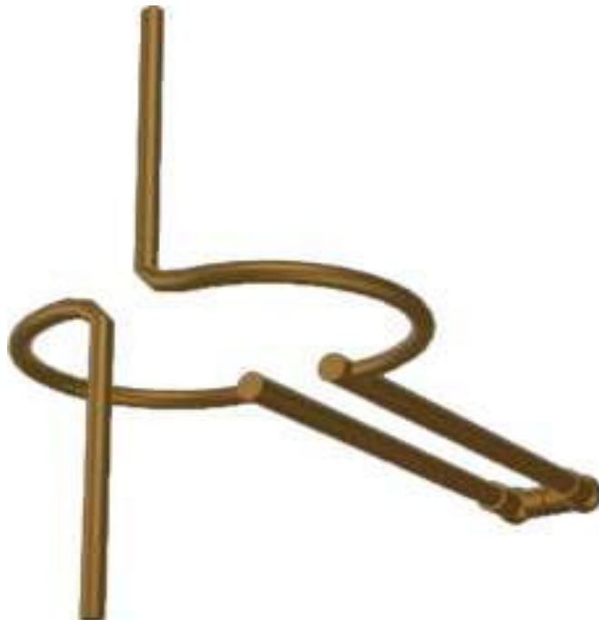
Fig 3.2d: Tapered helical or conical-spiral (forward-fire) Cp antennas
