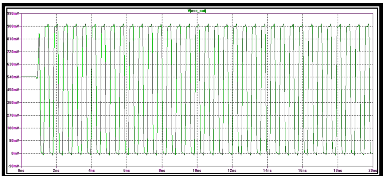
Figure 3.18: Observation of the frequency at VDD (-10%) while V_{in}=1
