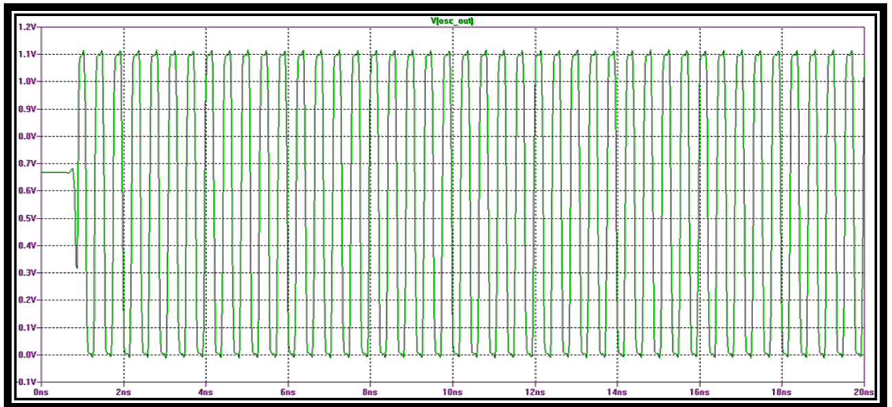
Figure 3.17: Observing the frequency at VDD (+10%) while V_{in}=1
