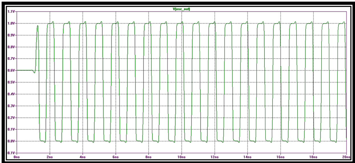
Figure 3.21: Output waveform of CSVCO due to process scattering.
