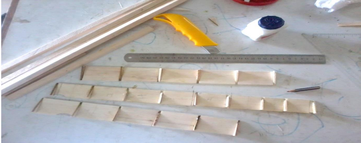
Figure 5.2: fabrication of control surfaces
