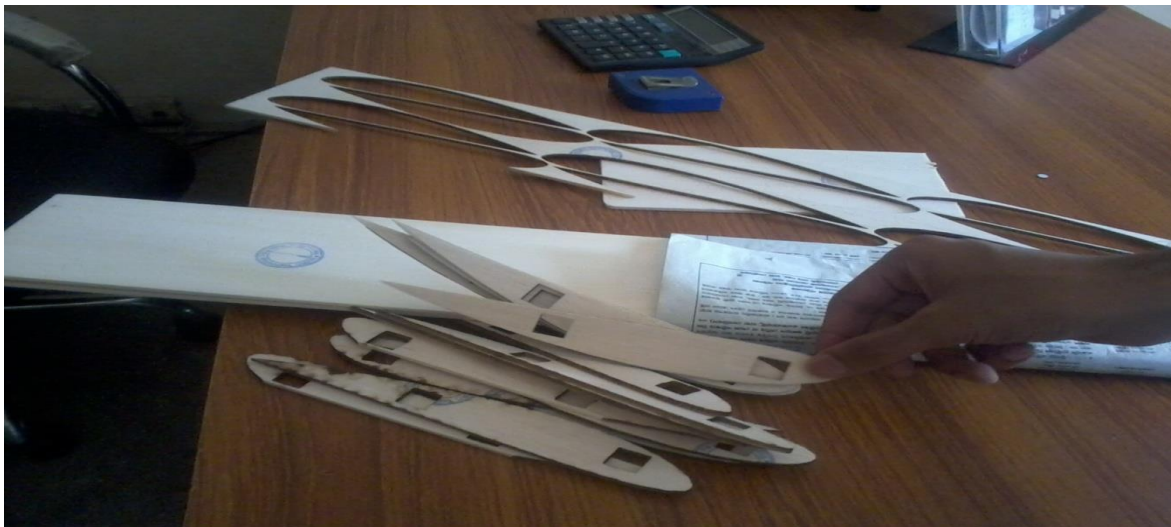
Figure 4.1: Cutting of ribs according to design specifications.
