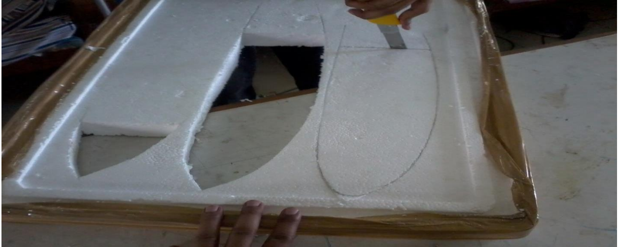
Figure 4.4: Cutting of polystyrene (cork sheet).
