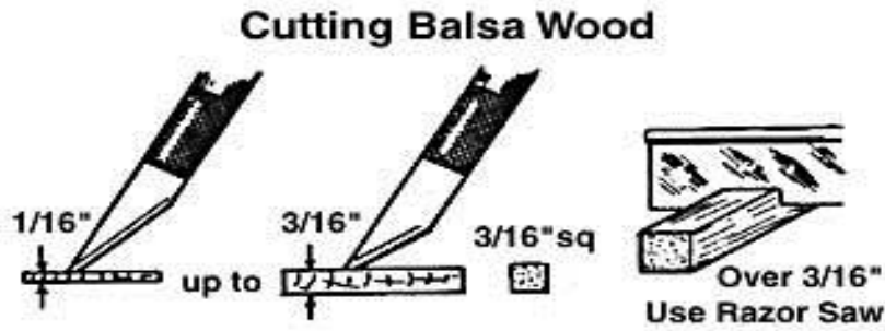
Figure 4.5: Balsa cutting procedure
