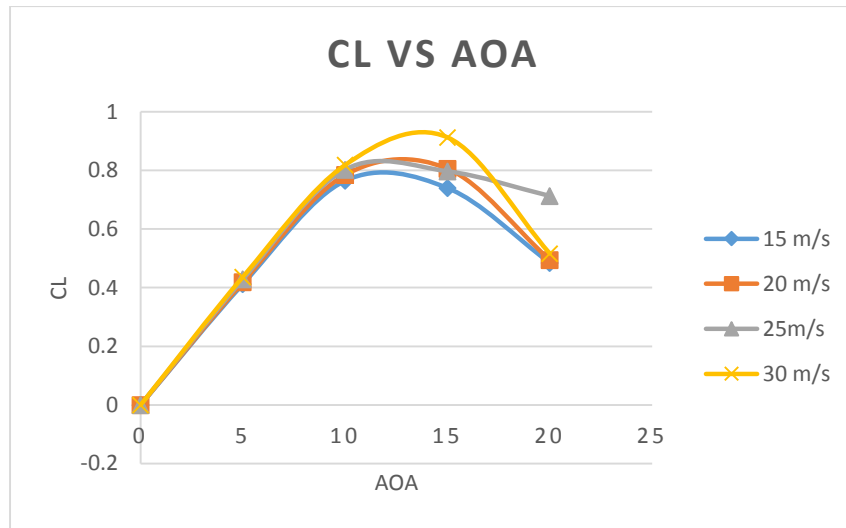
Figure 4. 5 Comparative CL Vs AOA graph at different velocities
