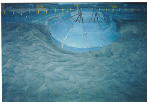
Fig 10. Local Scour around a Sloping Abutment
