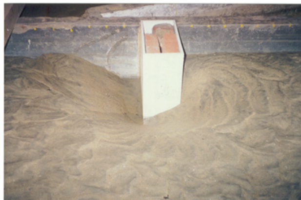
Fig 8. Local Scour around a Vertical Abutment
