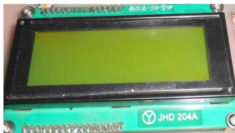
Fig. 5.10 LCD display from JHD
