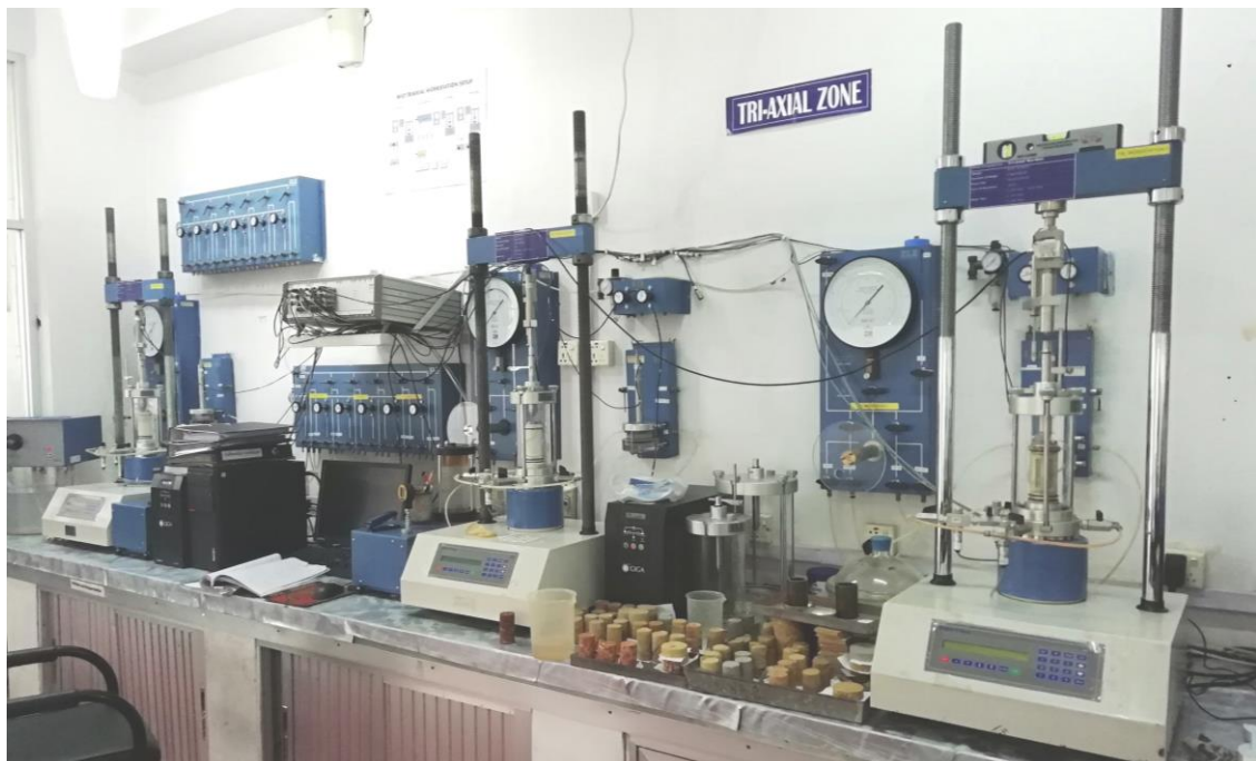
Figure 3.3 triaxial test in progress.
