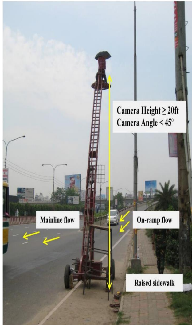
Figure 3.2 (h) Camera location on on-ramp showing details of the data collection process
