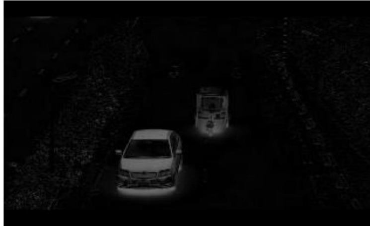
Figure 3.3 (c) The differential image (D) of frame I
