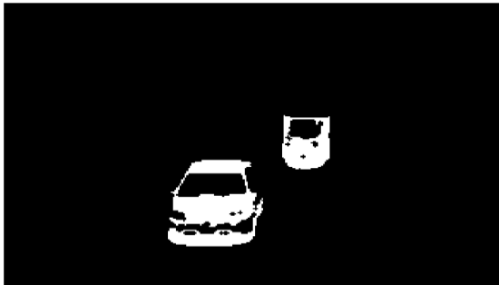
Figure 3.3 (e) Binary image after applying opening
