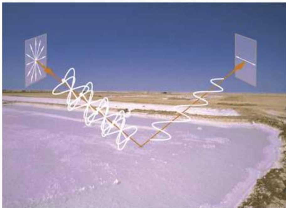
Fig 1.8: Polarization from reflection.
