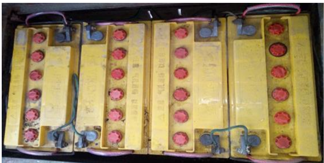
Fig 2.6: Lead acid battery of an Electric Rickshaw.
