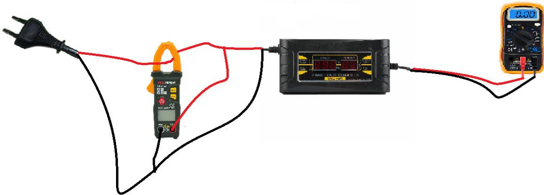
Fig 3.5: Arrangement of equipment for no-load test.
