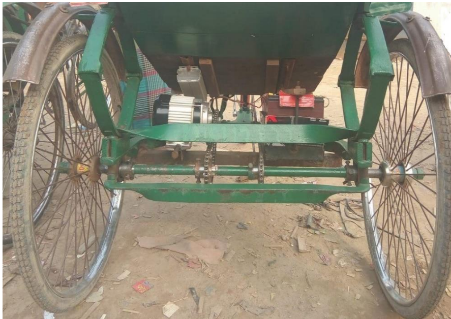
Fig 2.1: Electric Rickshaw (a) Side View (b) Motor and Battery parts.
