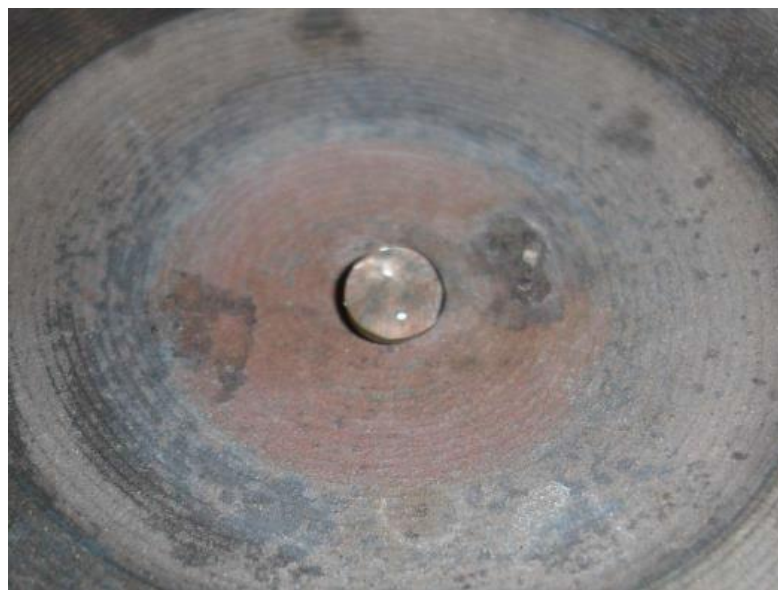
Figure 2.3: A water droplet experiencing Leidenfrost effect on a hot stove plate
