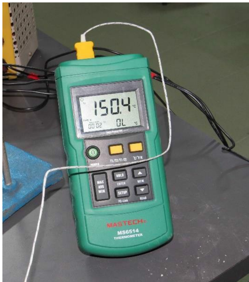
Figure 3.9: K Type Thermocouple Meter
