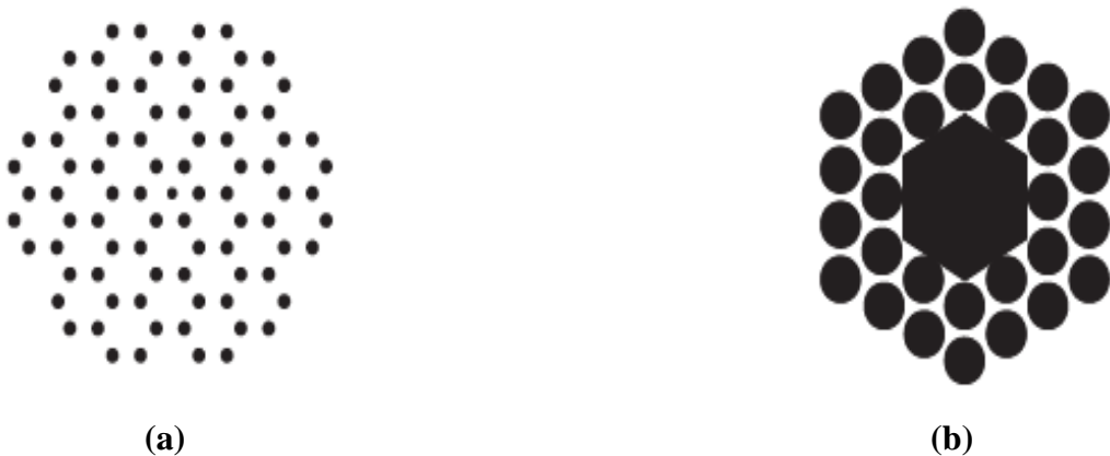
Fig. 1.15: Photonic band-gap (PBG) fiber structures in which the dark areas are air (lower refractive index) and the lighter area is the higher refractive index: (a) honeycomb PBG fiber; (b) air-guiding PBG fiber [2]
