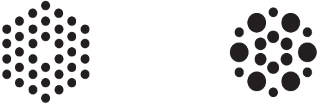
Fig. 1.14: Two index-guided photonic crystal fiber structures. The dark areas are air holes while the white areas are silica [2]
