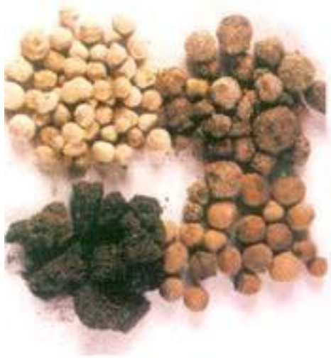
Figure 2.14: Pelletized and sintered fly ash makes a good lightweight aggregate.
