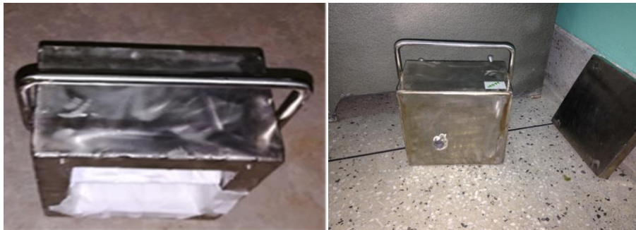
Fig. 3.5: Fabricated Lead Box for Shielding Camera
