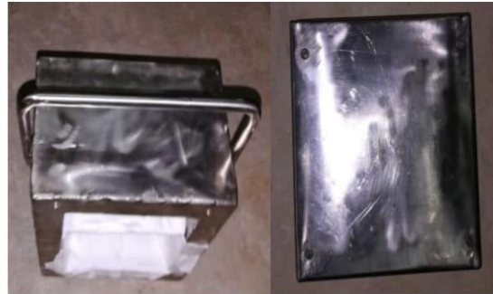
Fig.2. Lead Box with Stainless steel frame
