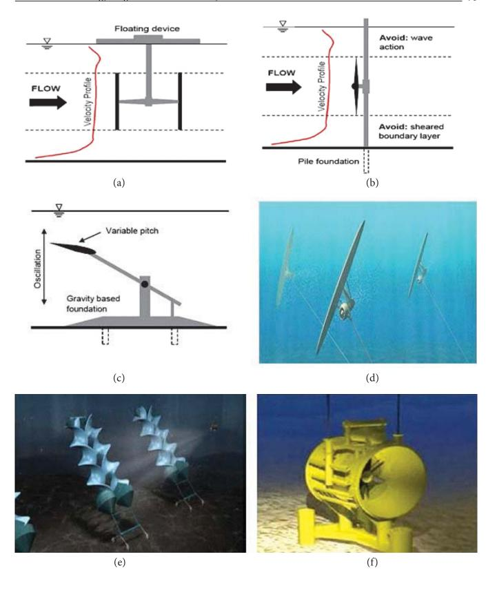
Fig 1. Different types of available turbine technologies (a) Vertical axis turbine, (b) Horizontal axis turbine, (c) Oscillating hydrofoil turbine, (d) Tidal kite, (e) Helical screws, and (f) Enclosed tip.
