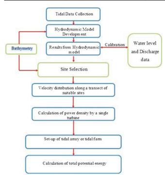
Fig 3. Flowchart presenting step-wise methods followed for tidal current power potential calculation.
