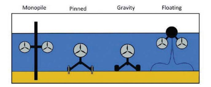
**Fig 2.** Types of foundation generally used for tidal energy converter.
