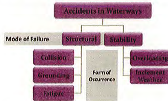
Fig. 2: Mode of failure and form of occurrence of accidents in waterways
