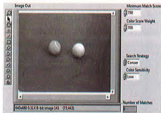
Fig. 6: Calibration for white ball may not work on green or black background
