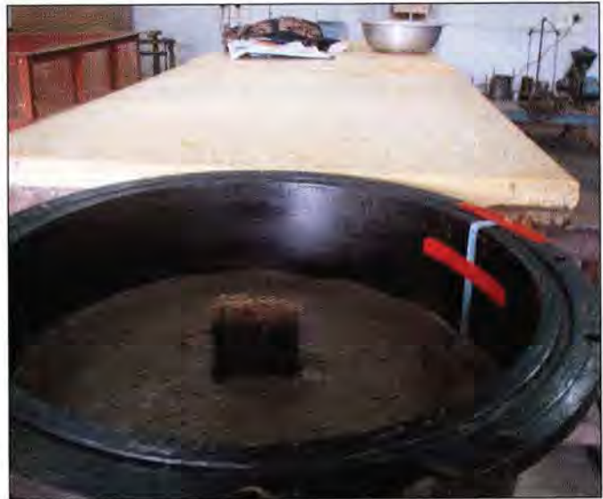
Figure 5: Steel Tank Filled with Soil Slurry (Test with Jute PVD)
