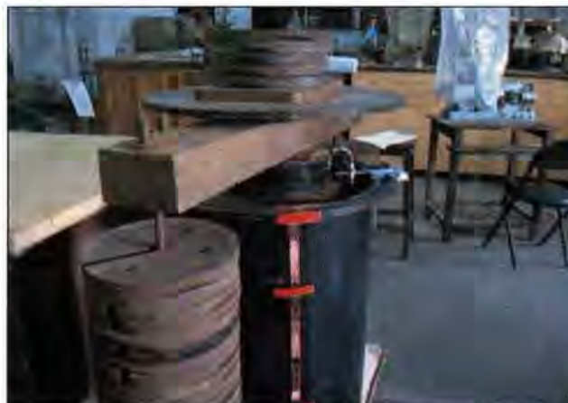
Figure 3: Soil Being Settled without Vertical Drain.
