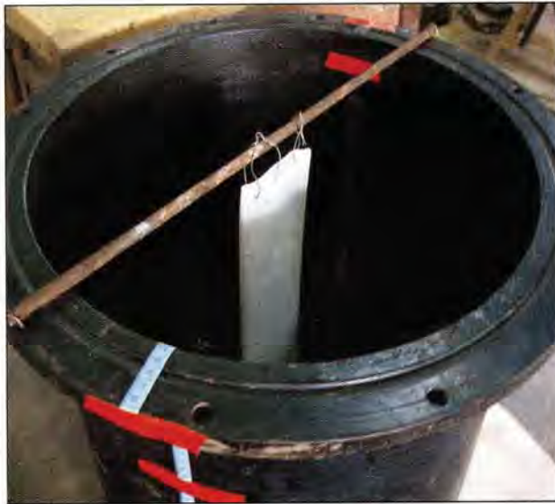
Figure 4: Synthetic PVD Hung before Pouring the Slurry
