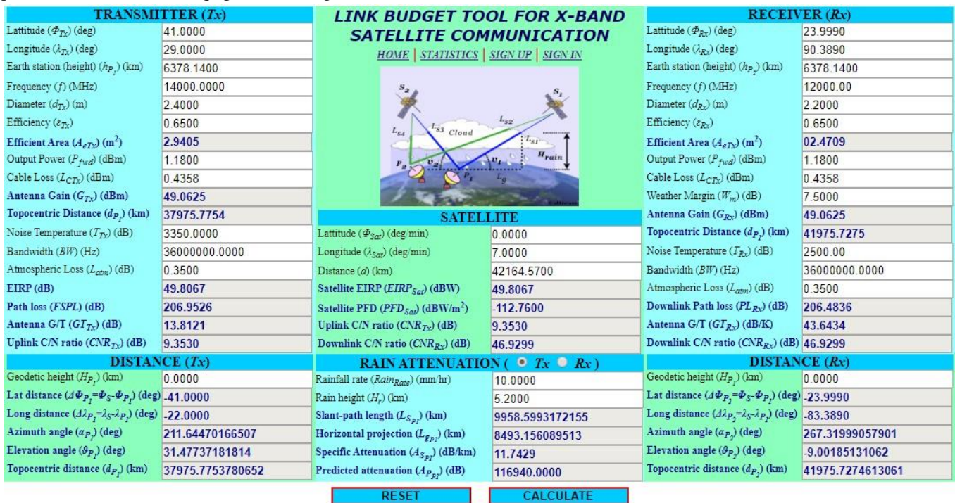
Figure 14: User interface of the proposed Link Budget Tool with six sections: TRANSMITTER (Tx) Earth Station, SATELLITE (Celestial Body), RECEIVER (Rx) Earth Station, DISTANCE (Tx), DISTANCE (Rx), and RAIN ATTENUATION (Tx and Rx). The highlighted texts and values are indicating the output parameters which cannot be changed while the un-highlighted texts and values are the input parameters that can be changed on demand.
