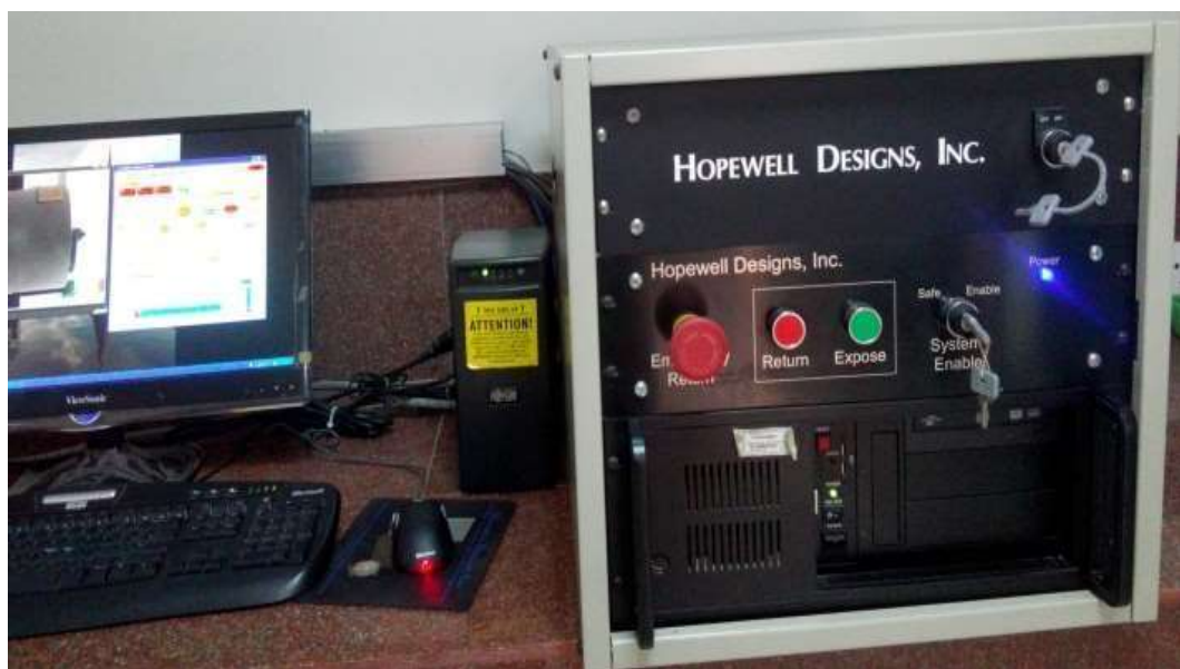
Figure 3.19: The Control panel system of Gamma Calibrator
