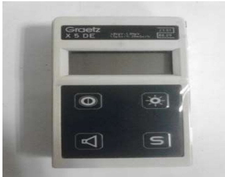
Figure 3.8: Graetz Survey Meter
