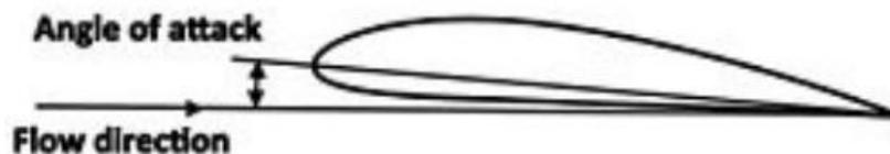
Figure 2: Angle of attack
