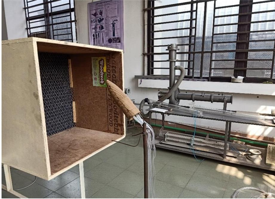
**Figure 7:** Experimental setup of 57 mm projectile for measuring static pressure.
