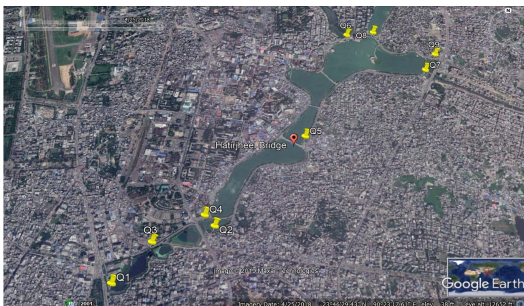
Figure 3.4: Major wastewater intrusion points in Hatirjheel Lake [45]
