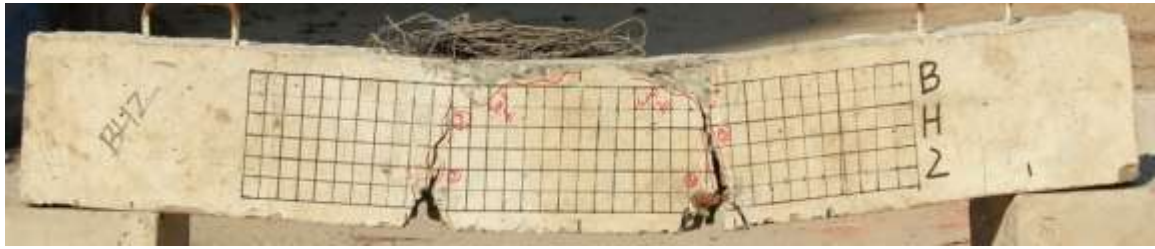
Fig 4. 5: Failure Mode for beam SSL-1 due to concrete crushing
