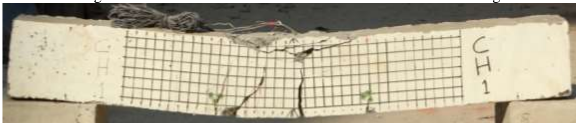
Fig 4. 7: Failure Mode for beam MSL- 1 due to concrete crushing
