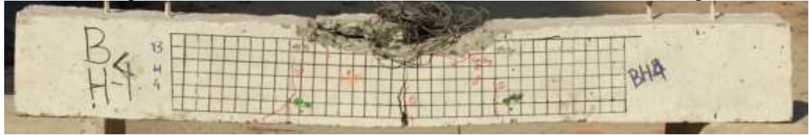
Fig 4. 14: Failure Mode for beam SSM- 2 due to concrete crushing
