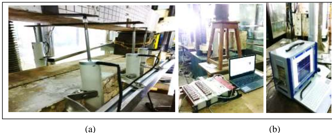
Fig 3. 11: (a) LVDTs' locations, (b) Data acquisition device, and channel box
