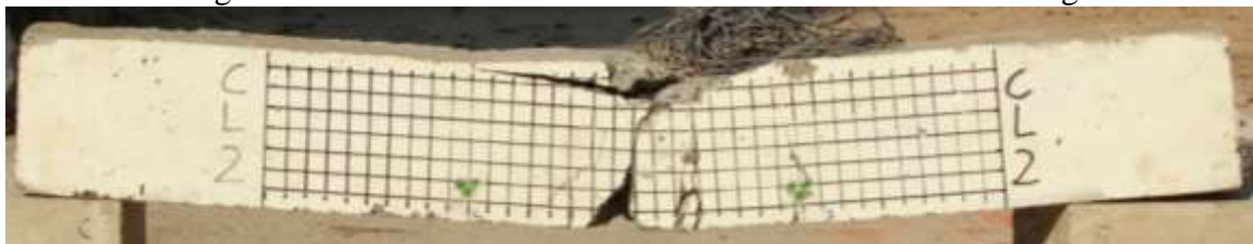
Fig 4. 6: Failure Mode for beam SSL-2 due to concrete crushing
