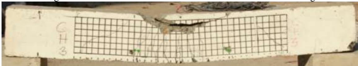
Fig 4. 27 : Failure Mode for beam MSH- 2 due to concrete crushing
