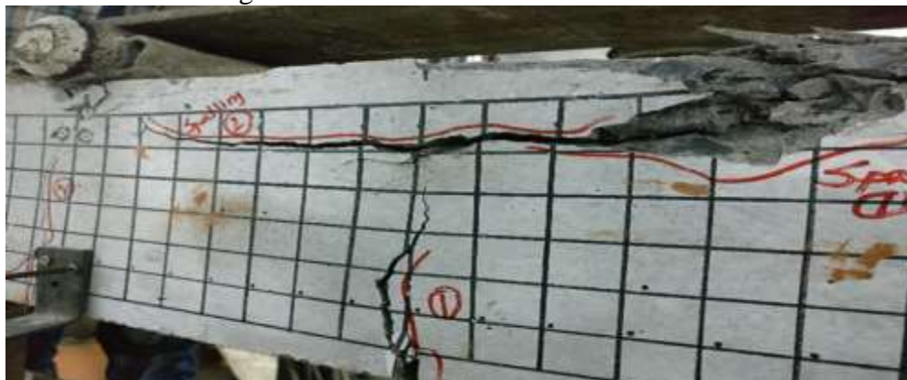
Fig 4. 10 : Crack Pattern for beam SSM-1
