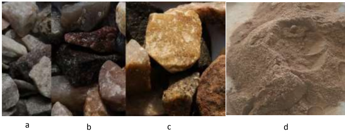
Fig 3. 1 : Types of aggregate used in research, here (a) 1/2" passing and 1/4" in retained, (b) 3/4" passing and 1/2" in retained, (c) 1" passing and 3/4" retained, (d) Stack of Sylhet Sand
