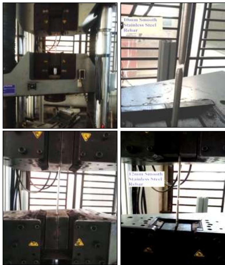
Fig 3. 5 : Photographs of Tensile Strength Test ASTM A955
