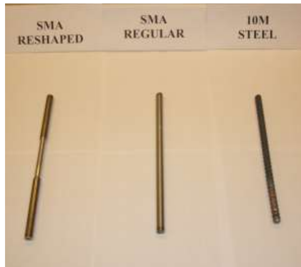
Fig 2. 4: SMA and conventional reinforcement samples. Adopted from Cramer, Covino Jr et al. (2002) [17]
