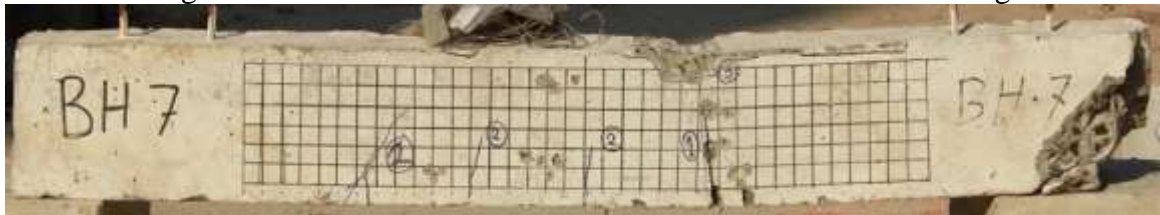
Fig 4. 14: Failure Mode for beam SSM- 2 due to concrete crushing
