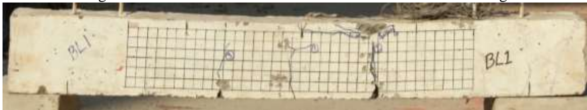
Fig 4. 5: Failure Mode for beam SSL-1 due to concrete crushing
