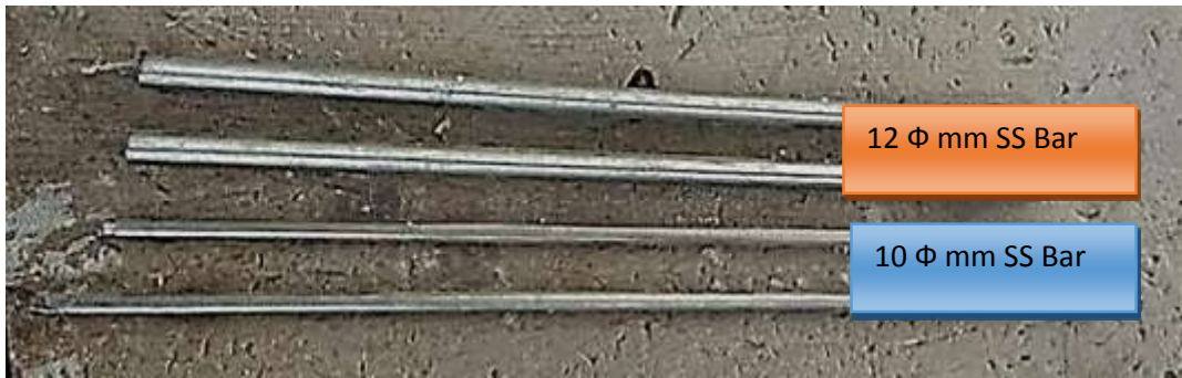
Fig 3. 4 : Plain Steel Stainless Steel Rebar samples
