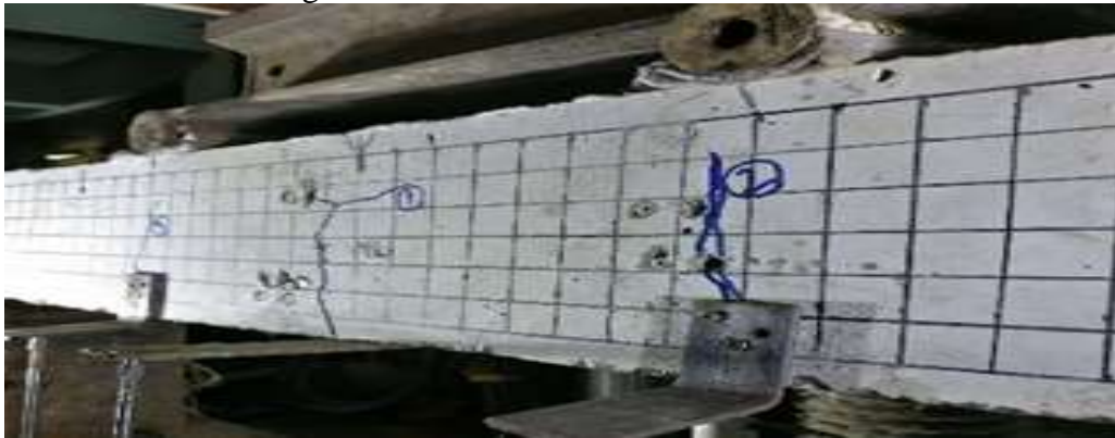
Fig 4. 17 : Crack Pattern for beam SSH-1
