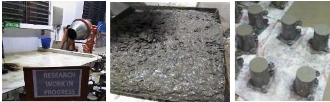
(a) (c) (b) Fig 3. 9 : (a) Casting Area (b) prepared fresh concrete and (c) Cylinder specimen
