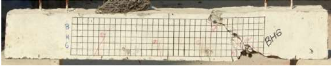
Fig 4. 23: Failure Mode for beam SSH- 1 due to concrete crushing
