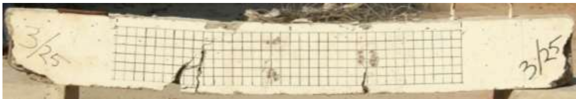
(a) Observed beam specimen
