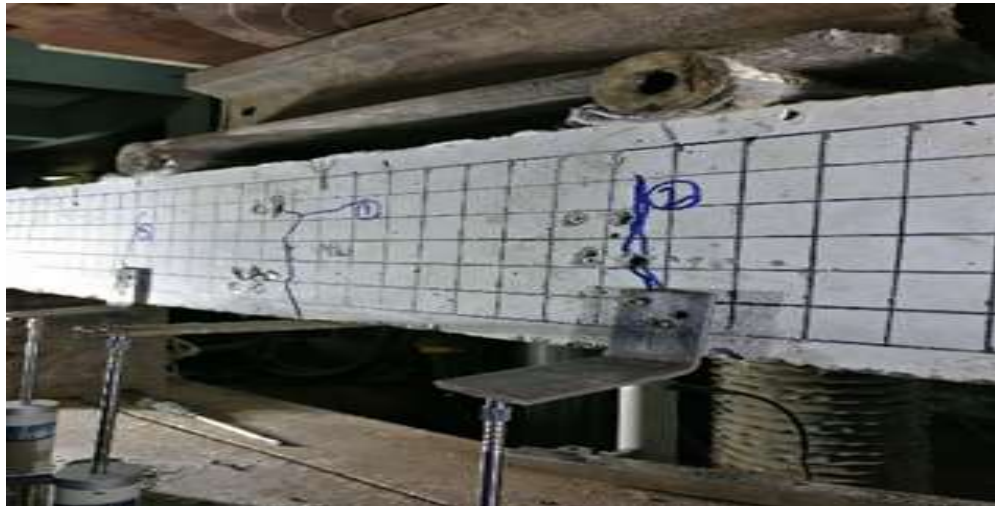
Fig 4. 12 : Crack Pattern for beam SSM'-2
