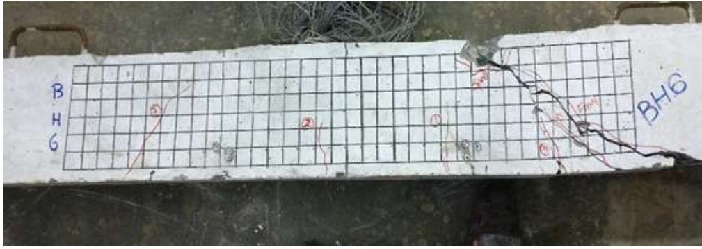
Fig 4. 17 : Crack Pattern for beam SSH-1
