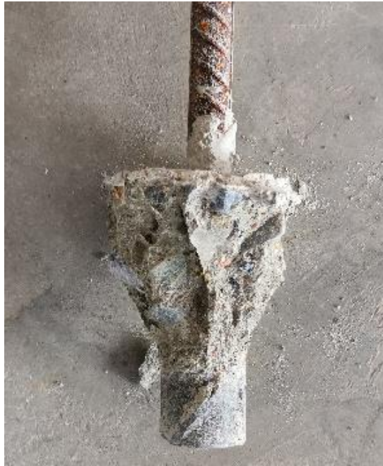
Figure 4. 18: Concrete conic frustum after cast in pull out test of rebar.
