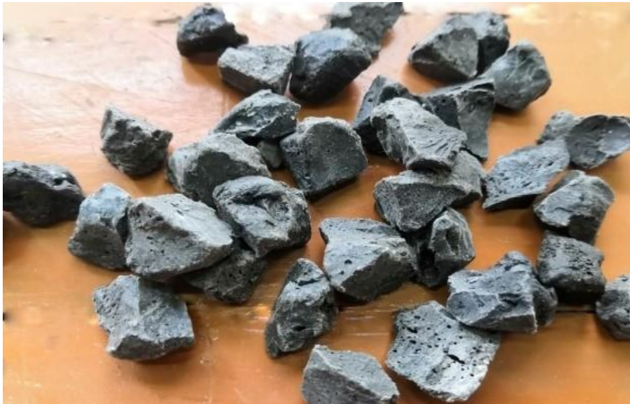
Figure 1. 1: Processed Polypropylene (PP) aggregate
