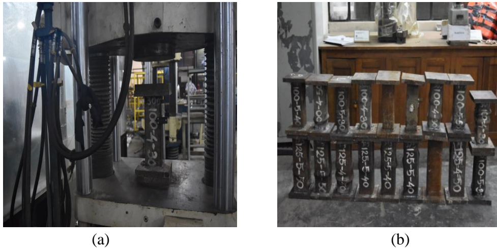
Figure 3.14 (a) Setup of concentrically loaded stub columns (b) sample stuck after test
