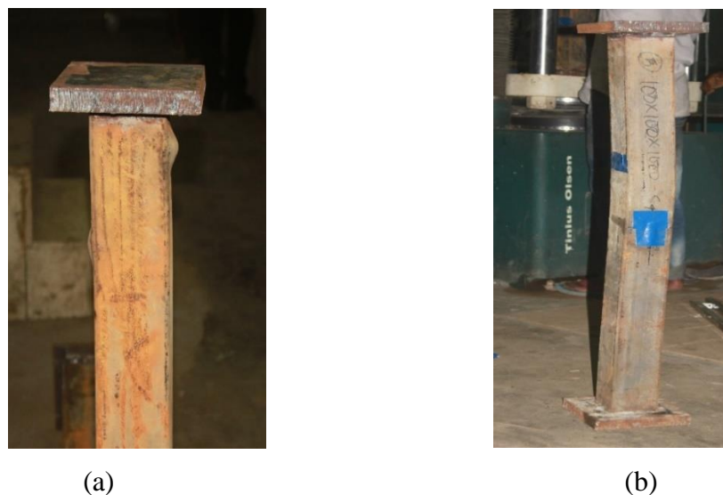
Figure 4.22 After test of CFST column (a) without fiber (b) with fiber
