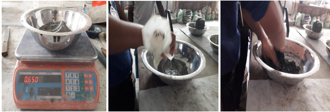
a) Weighing cement
