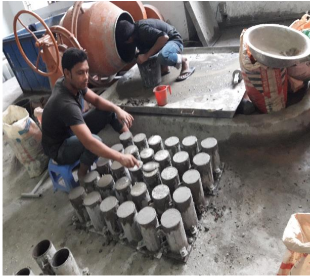
Figure 3.14: Photographs of sample preparation for compressive strength of cylindrical concrete specimens
