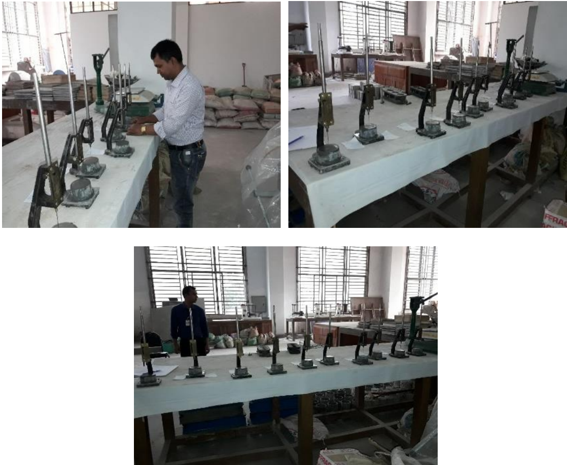
Figure 3.9: Photographs of sample test set-up for setting time test
