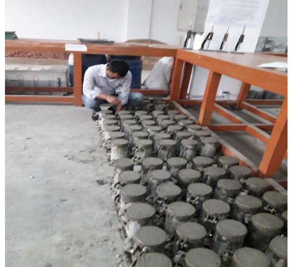
Figure 3.14: Photographs of sample preparation for compressive strength of cylindrical concrete specimens
