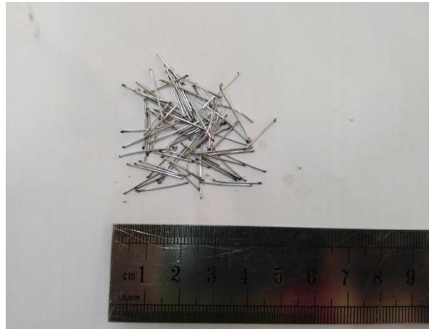
Figure 3-4: GI fiber of 0.51 mm diameter
