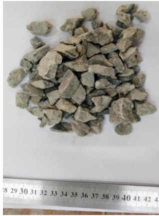
Figure 3-1: Crushed stone chips
