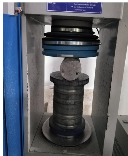
Figure 3-10 : Tensile strength test of concrete cylinder
