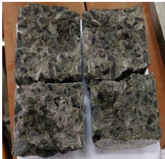
Figure 4-12: Columnar failure of NAC without GI fiber
