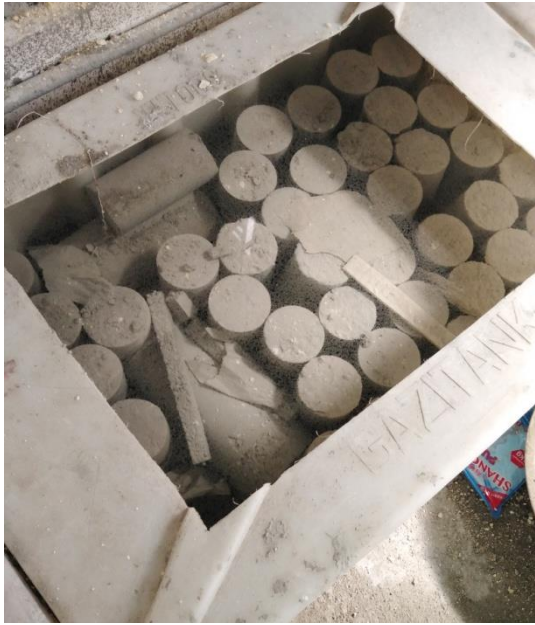
Figure A.3: Curing of Samples
