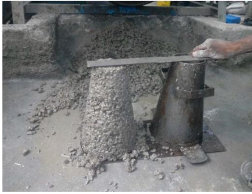
Figure 4-1: Slump test of concrete mixes
