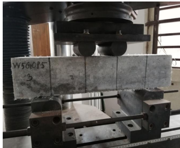
Figure 3-11: Test set up for quasi-static flexural test
