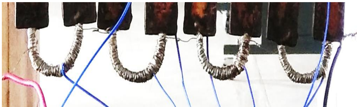
Fig.3.1.4.3: Heating coils at evaporator section
