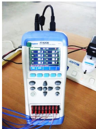
Fig.3.1.5.1: Temperature data logger.
